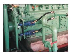
T100-B dual starter mounted on a Worthington *SL-10. Simple installation, power and reliability* make the T100-B ideal for starting engines up to 300 liters.
