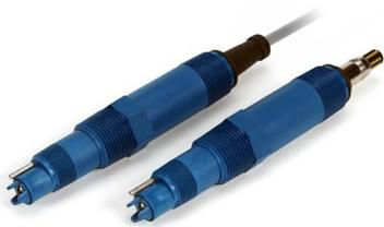
The Rosemount 3900 and 3900VP General Purpose pH/ORP Sensors feature a chemically resistant Ryton plastic body, along with a built-in solution ground for advanced diagnostics and a Pt-100 RTD for temperature compensation. These sensors are available with either an integral cable connection (3900) or Variopol (VP8) connector (3900VP). Variopol cables are sold separately (see [Accessories](#)).
