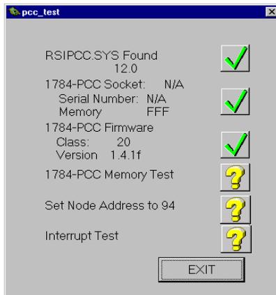
The 1784-PCC installation test utility automatically looks for your card and begins the tests. As the tests are completed, a green check mark appears, illustrating that the particular test was successful.
